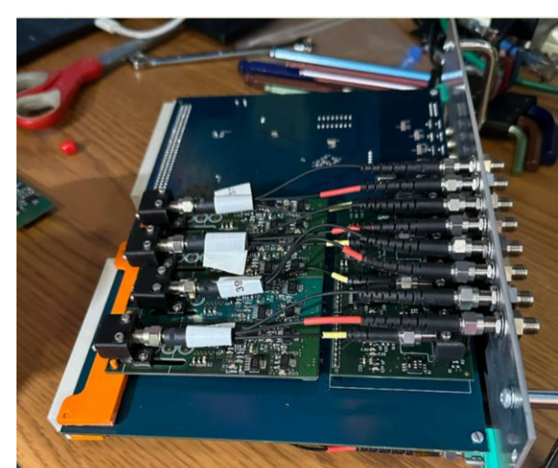
Fig. 4 - Board from DAQ Rack, showing the LED on left part of the board, as well as cables which connect to the monitoring PMT and inside the experiment.
