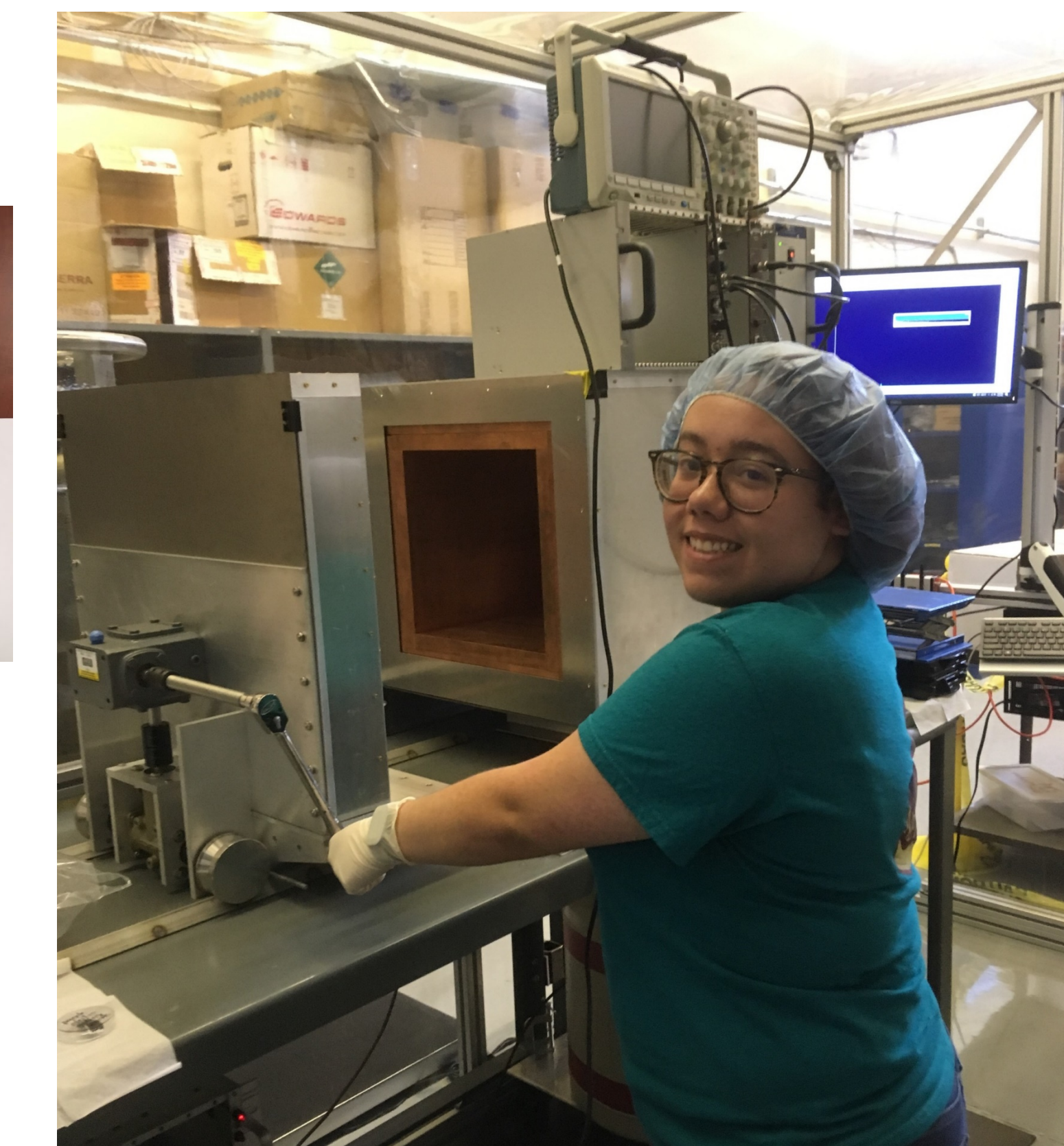
Fast loading bottled samples into the 2 ton shielded Rabbit Ge-detector chamber for \gamma -ray assay
