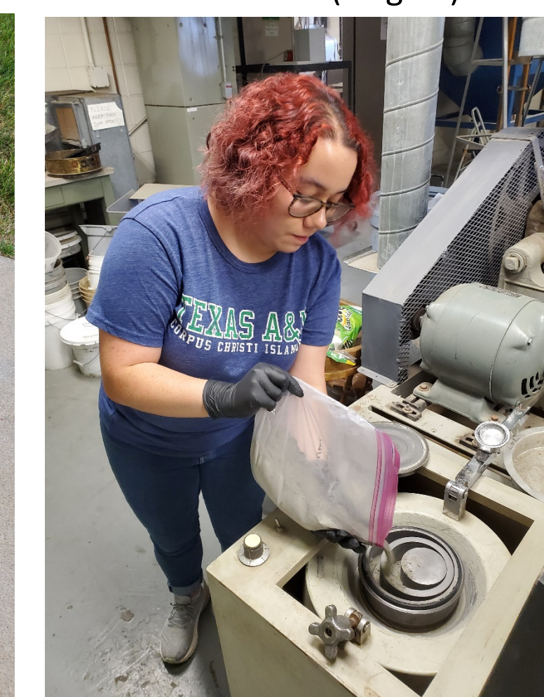
Fine rock crusher (stage 2):
