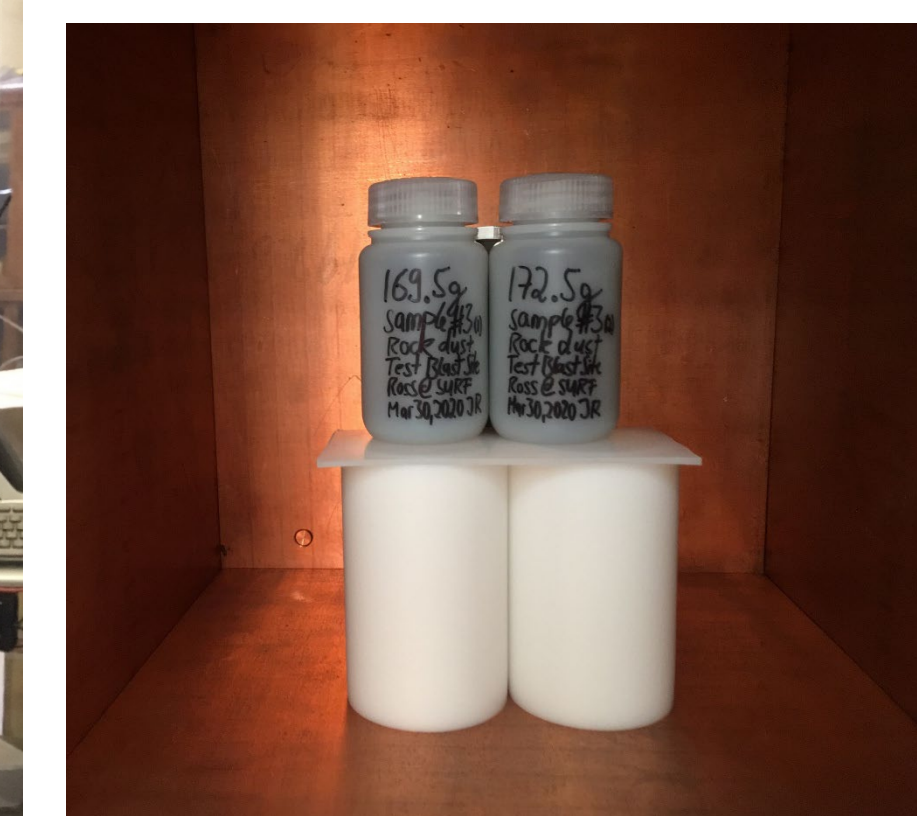
Re-measured bottled samples from the DUNE test blast site inside the Rabbit Ge-detector's assay chamber
