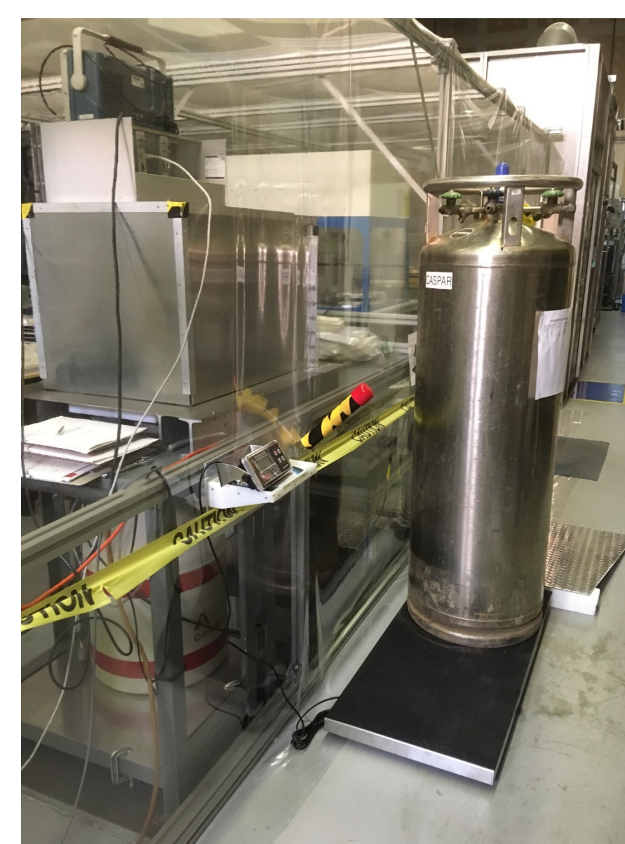
Other side view of LN2 dewar with Ge-detector in view.
